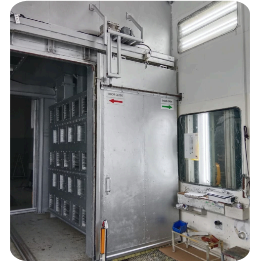
CONVERT TO AUTOMATIC SLIDING DOOR WITH PLC LOGIC
