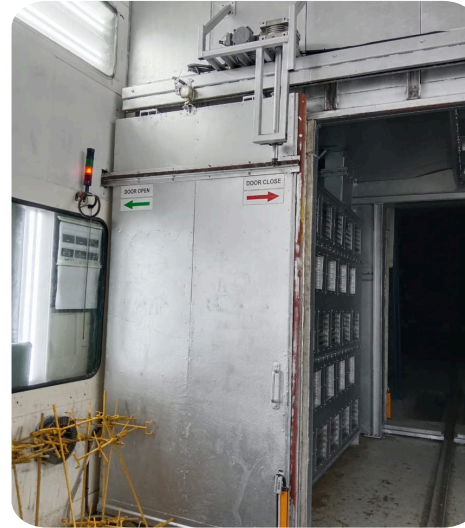
CONVERT TO AUTOMATIC SLIDING DOOR WITH PLC LOGIC
